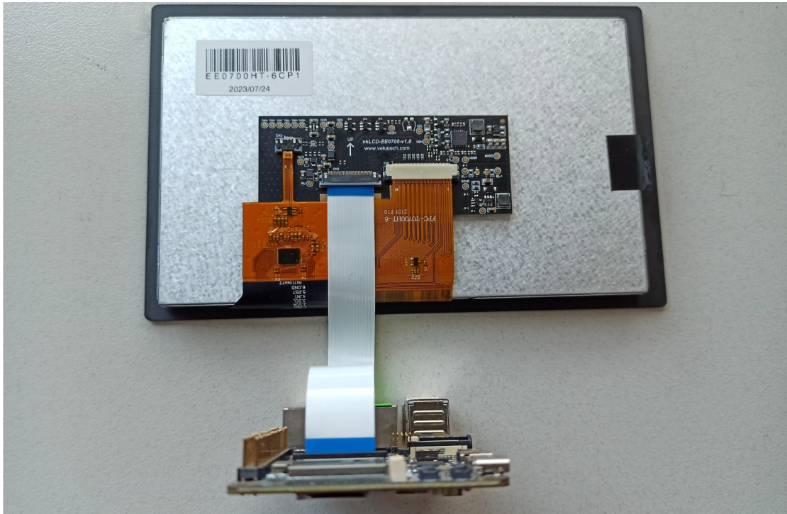
vkcrz-dsi-vklcd-ee0700 display FPC cable orientation
